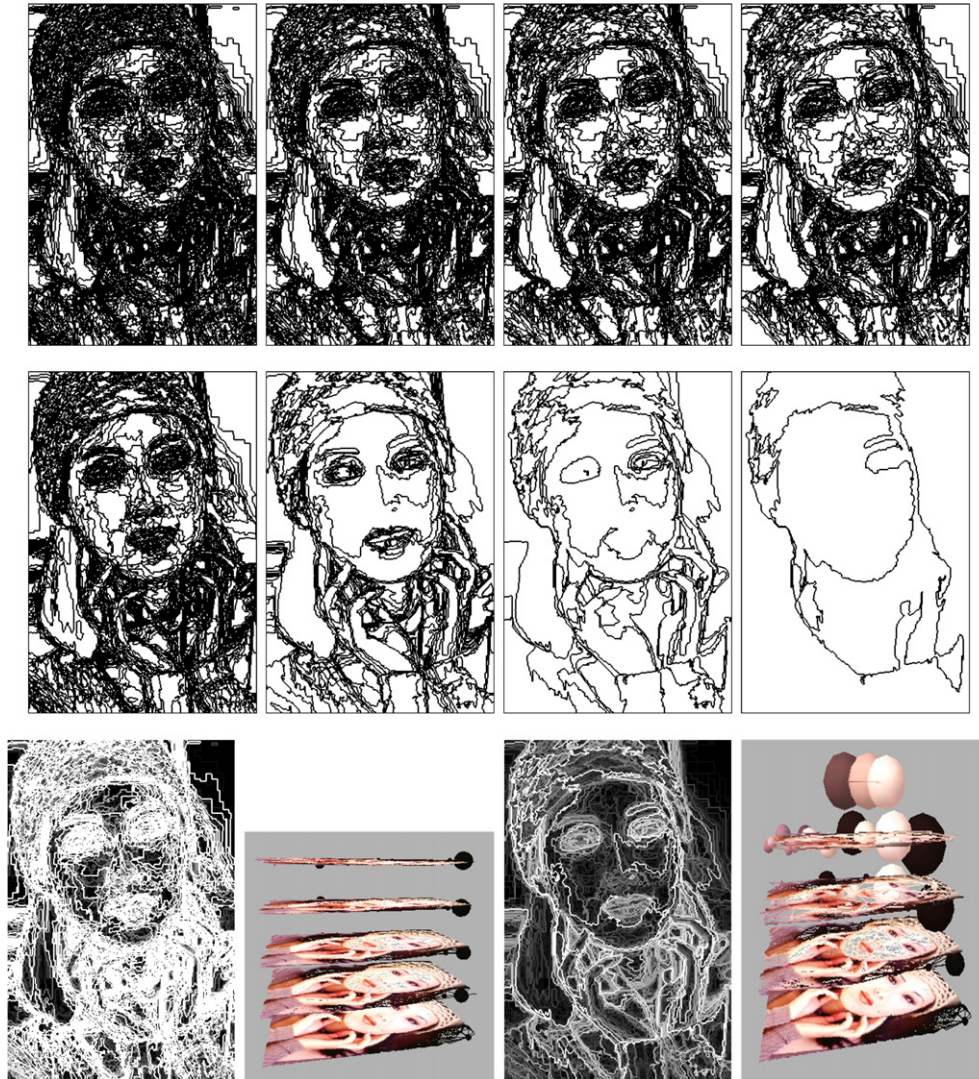
Fig. 11. Multi-scale segmentations in a hierarchy of partitions for scales 5, 10, 15 and 20 (columns 1–5) with two different merging criteria: fixed threshold (first row) and adaptive threshold (second row). Third row, columns 1 and 3 show the saliency map of the produced hierarchy. Third row, columns 2 and 4 present a hierarchical view of the region adjacency graphs. Hierarchies were obtained on Fig. 9(d) with the fine partition of Fig. 9(e).
